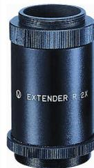
Tele-Extenders extend the effective focal length of the optical system. They can be used in place of a Barlow lens for imaging applications. Extends the focal length of the R150S from 750mm to 1500mm (f/10) and the R130S from 720mm to 1440mm (f/11).
