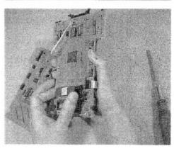
The pins on the new EPROM may be slightly spread apart. If they are, straighten them out as follows before inserting them into the chip socket.
