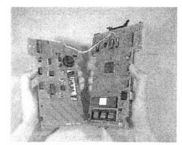
Loosen the old EPROM from the chip socket by using the flat screwdriver to alternately lift the EPROM at both ends using twisting motions.
