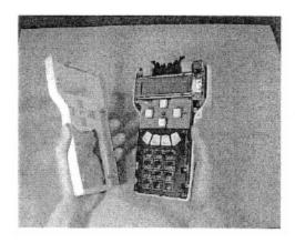
Remove four tap screws at the positions indicated on the illustration using the Phillips screwdriver.
