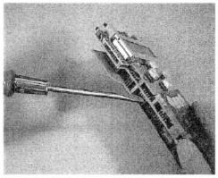
Separate the upper and the lower circuit boards.
