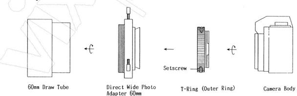
Attach the T-Ring to the Direct Wide Photo Adapter 60mm and lock it with the setscrews.
