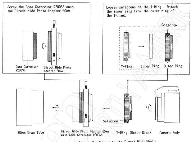
Attach the T-Ring to the Direct Wide Photo Adapter 60mm and lock it with the setscrews.
