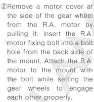
(Note: If the gear wheels are engaged too tightly. The motor may not operate and may go wrong.)
