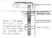
Tighten the Decl. motor fixing bolt with the wrench (5mm size).
