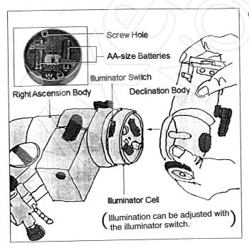
2 Load two AA-size batteries into the illuminator cell. After loading the batteries, make sure that the light can be on. Place the illuminator cell between the right ascension body and the declination body. Screw the declination body and the illuminator cell to the right ascension body. If you have somebody hold the illuminator cell, it can be done with ease. (Note: The illuminator is not provided with the batteries.)
