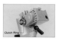
4 Connect the Decl. motor cord to the motor.
