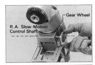
3Install the motor on the mount with the R.A. motor fixing bolt.
